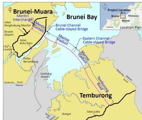
Fig. 1. Layout Plan of Temburong Bridge Project
