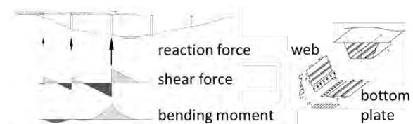
Figure 1. Schematic representation of the loading over the launching bearing [11] and [1].
