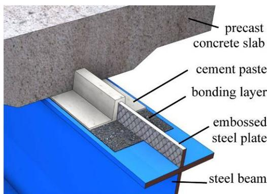
Fig. 1 *General view of a connection by adherence*
