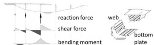
Figure 1. Schematic representation of the loading over the launching bearing [1].
