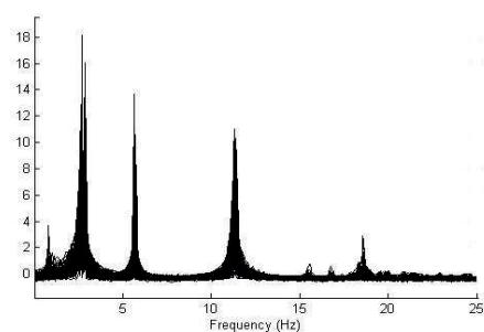
Fig. 2: The vibration modes of the bridge
