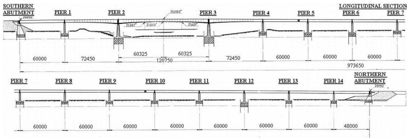
Fig. 1: Longitudinal section of the bridges across the Low-Rhine.
