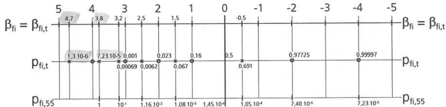
Fig.1: Reliability index  $\beta_{fi}$  as a function of the probability  $p_{fi,55}$  of getting a fully fire engulfed compartment during the life time of the building.
