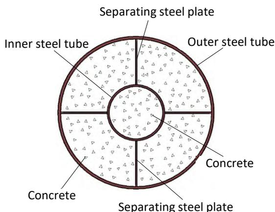
Figure 1. Cross section of multi-cell CFT column with double-layer circular steel tubes
