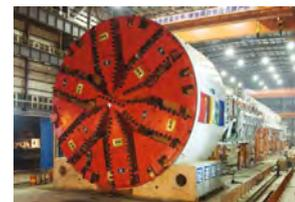
Fig. 2: Front shield of a TBM
