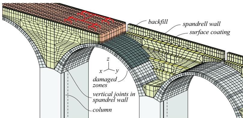
*Fig. 2: View of the 3D FE-model.*
