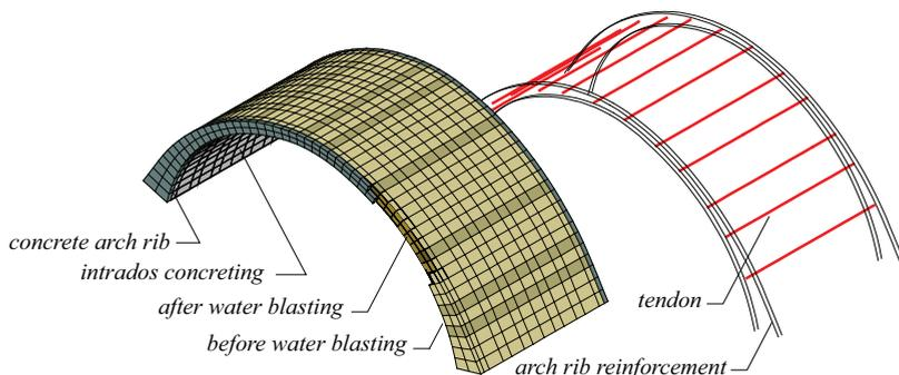
*Fig. 3: View of the 3D FE-model for modelling of strengthening stages.*
