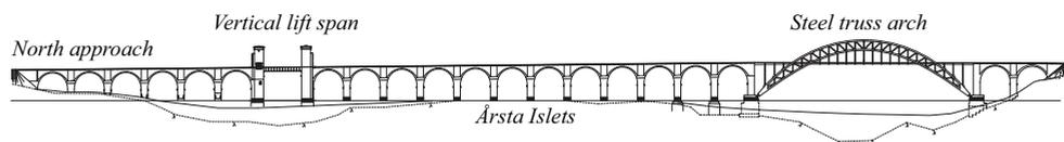
*Fig. 1: Elevation of the old Årsta railway bridge.*
