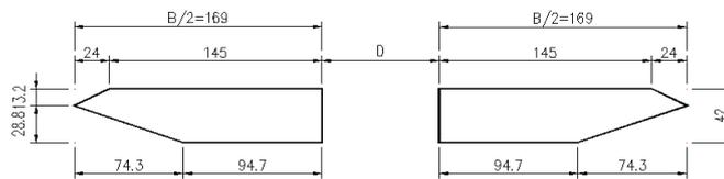
Fig.2: Girder sections of wind tunnel test.(unit:mm)
