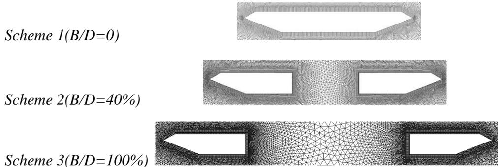
Fig.3 Local mesh of three numerical simulation model
