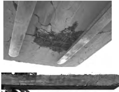
Figure 3: Fibre concrete panel after blast
