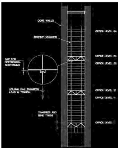
Figure 3: Robustness of primary trusses (Section E-W)
