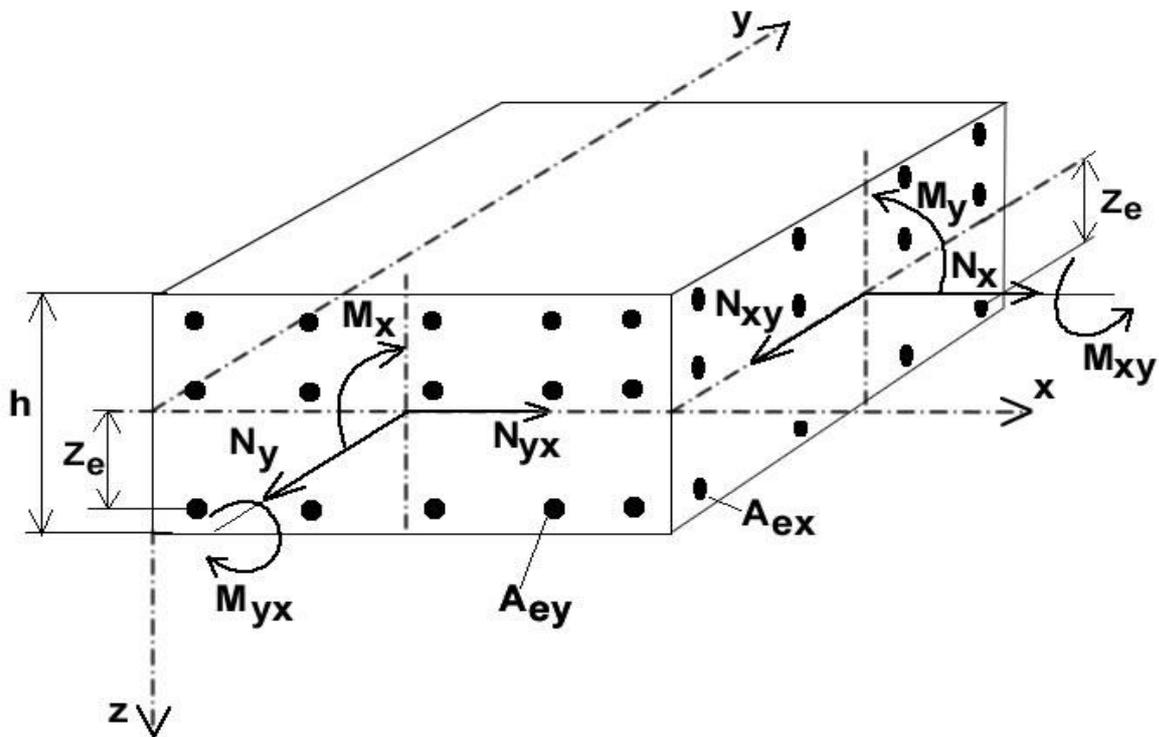
Fig. 1: Slab Element
