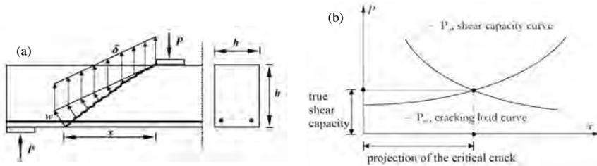
Fig. 1: (a) formation of diagonal crack followed by sliding failure, (b) shear capacity determined by intersection point of  $P_{cr}$ -curve and  $P_u$ -curve.
