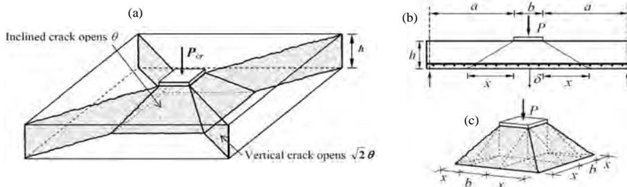
Fig. 2: Cracking mechanism and punching mechanism in a two-way spanning slab.
