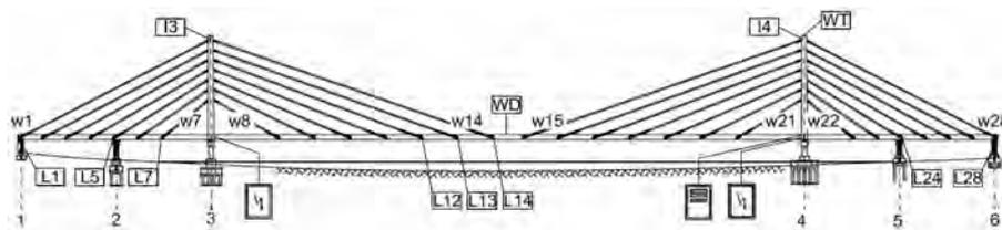
Fig. 2: The diagram of the bridge. The gauges: L1÷L28 – load cells, I3÷I4 – inclinometers, WD, WT – anemometers. The strain gauges are spread in the bottom of pylon (no.4) and superstructure.
