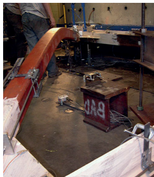
Figure 1. Inelastic brace buckling failure [1]
